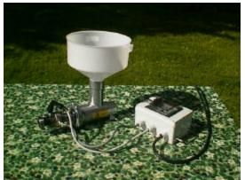
SKEPPSTA MASKIN AB Täby Skeppsta SE-70594 ÖREBRO. SWEDEN Oilpress Type 20 and electric aggregate box. 220 volt 50 Hz 1 phase Std.
