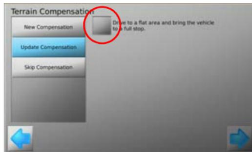
13. Turn the vehicle around through 180°, and stop in exactly the same position as before and tap the **grey square** button.
